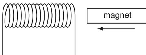
In which direction does the induced e.m.f. make the coil move?
