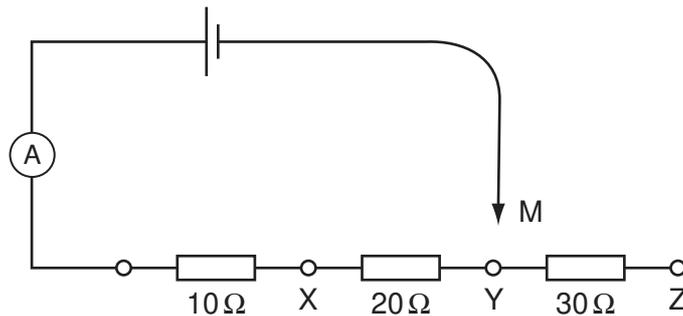
When M is connected to X, the ammeter reads  $0.6\ \text{A}$ .
