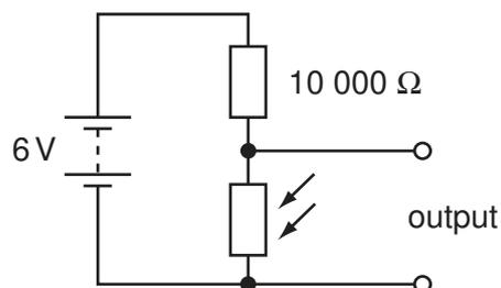
What should be the resistance of the LDR for the output to be 3 V?
